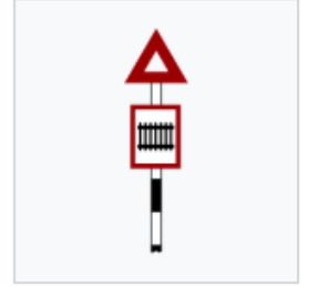
Guarded railway crossing
