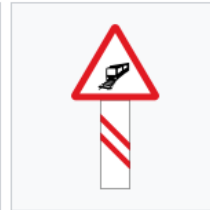
Unguarded railway crossing (200 metres ahead)
