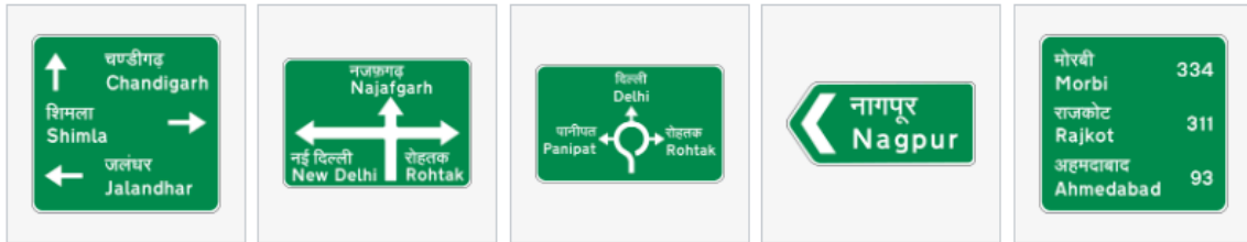
Stack-type advance direction sign
