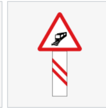
Unguarded railway crossing (200 metres ahead)
