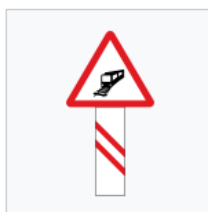
Unguarded railway crossing (200 metres ahead)
