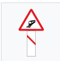
Unguarded railway crossing (50 - 100 Metres Ahead)
