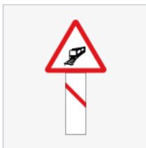
Unguarded railway crossing (50 - 100 Metres Ahead)
