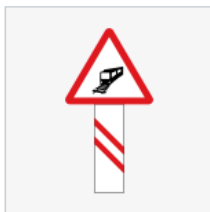
Unguarded railway crossing (200 metres ahead)
