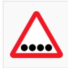
Blind persons likely on road ahead
