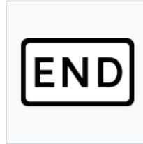
Supplementary plate "END" at the leaving side of work zone
