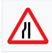
Reduced Carriageway Left Lane(s) Reduced
