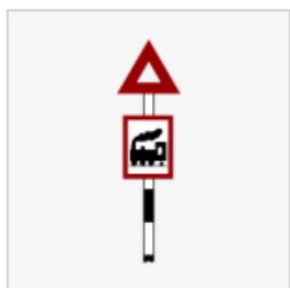
Unguarded railway crossing
