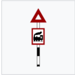
Unguarded railway crossing
